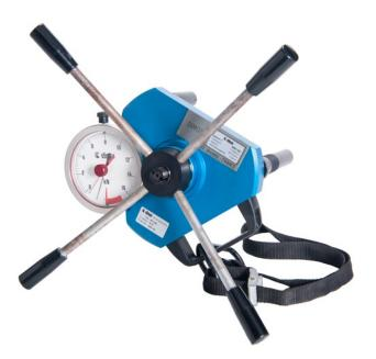
The extractometer is a control tool to check the traction resistance of the plugs.
